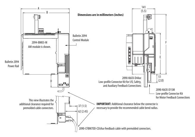
The AM power module is shown mounted to the power rail with the control module attached.
