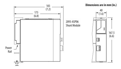
Modules are shown mounted to the power rail and the dimensions reflect that.
