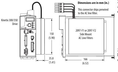
2097-F1 and 2097-F2 side-mount line filters add 35.8 mm (1.41 in.) to the width of your drive.
