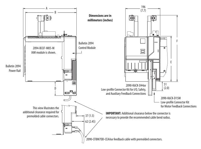
The IAM power module is shown mounted to the power rail with the control module attached.
