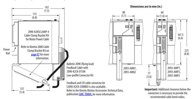
Modules are shown mounted to the power rail and the dimensions reflect that in the depth of the module.
