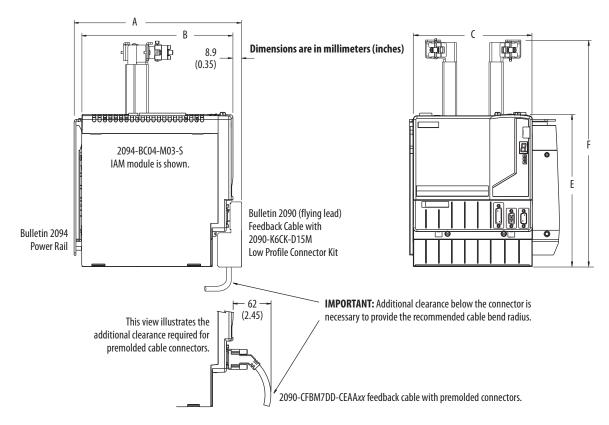
Modules are shown mounted to the power rail and the dimensions reflect that in the depth of the module.
