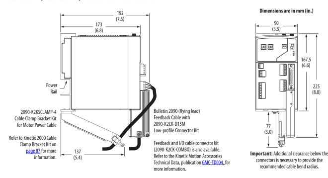
Modules are shown mounted to the power rail and the dimensions reflect that in the depth of the module.
