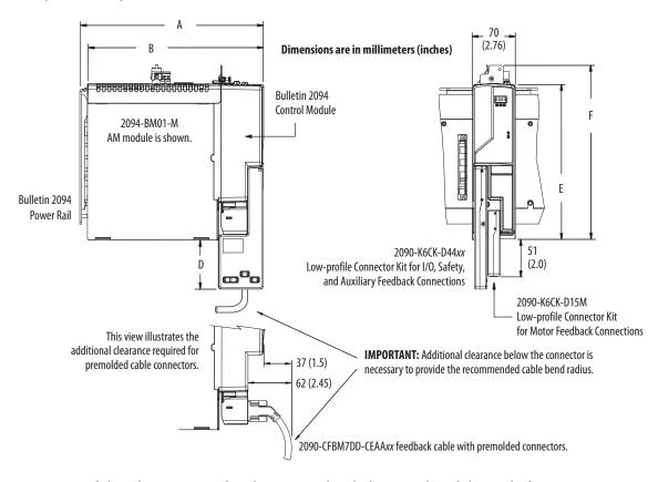
The AM power module is shown mounted to the power rail with the control module attached.
