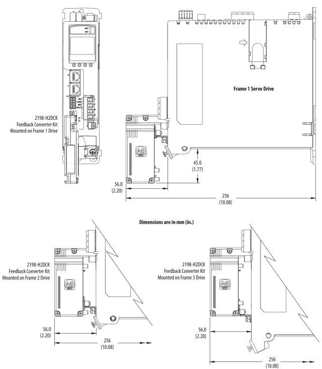
Refer to Hiperface-to-DSL Feedback Converter Kit on page 20 for motor/actuator compatibility and product dimensions.
