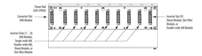
For example, the 2093-PRS1 power rail contains one inverter slot. This limits the use of this power rail to systems requiring only one inverter slot. Similarly, the 2093-PRS2 power rail contains two inverter slots. This limits the use of this power rail to systems requiring up to two inverter slots. When selecting a power rail, determine the number of inverter slots required by all rail-mounted modules and select one with that minimum number of inverter slots.
