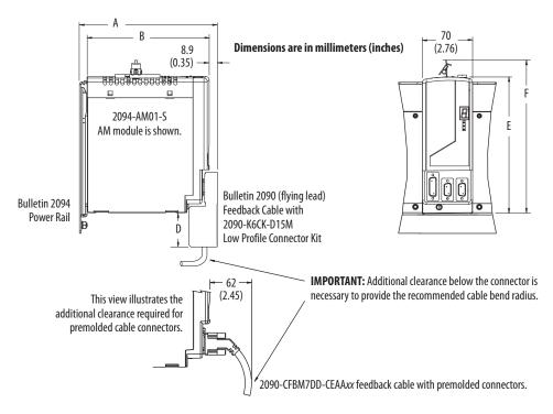
Modules are shown mounted to the power rail and the dimensions reflect that in the depth of the module.
