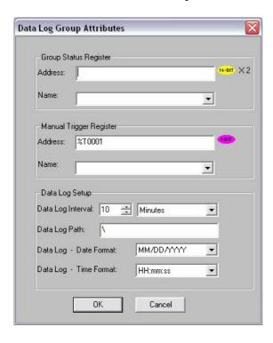
When Data Log Configuration is complete and downloaded to the target unit, the controller must be in RUN mode. The application will set the Global Enable Register bit to start the Data Log process (Always ON bit was set up as global trigger).
