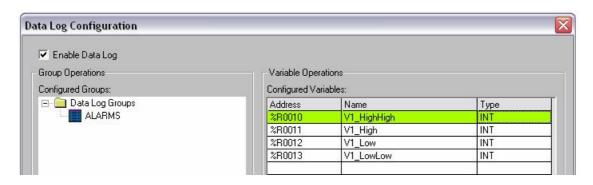
Data Log feature is designed to allow the application to periodically log register values to removable media. Registers can be organized in groups and every group can be configured separately. For the purpose of this Lab we are going to call it the **Auto Mode**.
