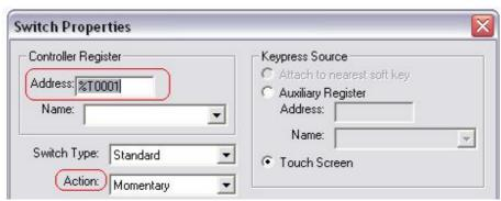
Specify an unused bit as a Controller Register and configure the action as Momentary.
