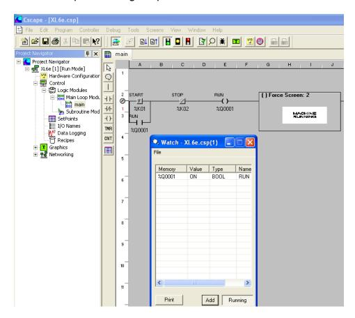
The Data type of a registers can be changed upon right click / Format on the register in the Data Watch.
