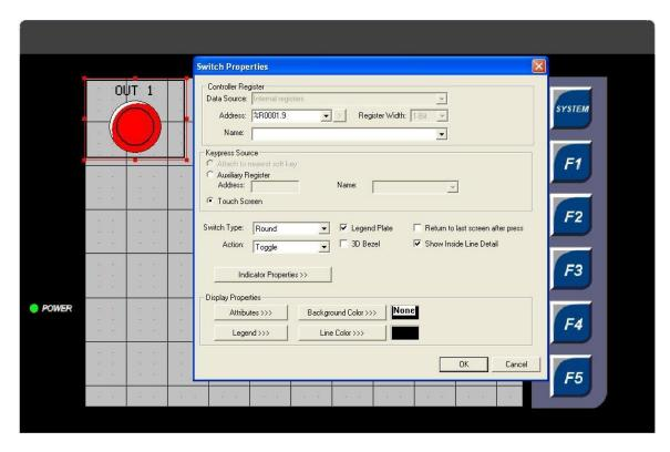
When the internal Registers are being used, then the OCS registers (%R0001) should be used. Save and Download the program to the OCS.
