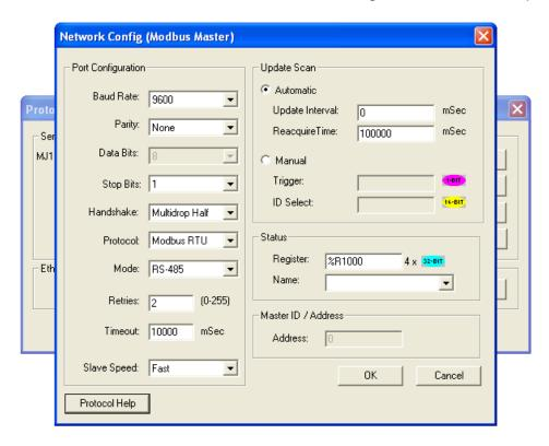
Enter the details required for the communication protocol. Protocol help button opens up the Modbus Protocol help. Click OK to save the settings.
