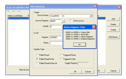
Data Mapping window opens up. This window helps us to configure the particular registers to be scanned during the communication from the particular device. Select the target device from the device name list. Bracketed number indicates the MODBUS Node ID.
