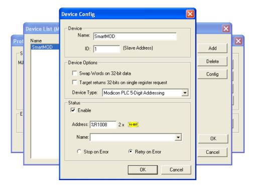
Enter the name and MODBUS ID for the device. Select the **Device Type** from the dropdown box and enable the Status. The status register provides the feedback of the connection, which can be useful for troubleshooting, if need arises.
